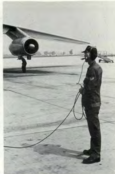
Left, top down, airman removing chocks must be aware of APU exhaust; checking flight controls with engines running; checking fasteners with engine running. Above, engine check with engine at high power setting; ground observer with microphone and earphones during engine check.
